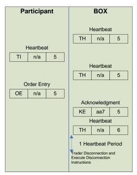
When the Participant connects, they specify the inactivity interval corresponding to the number of non-responded heartbeat messages (Message Type TH) the Exchange must count before disconnecting. A Heartbeat message can be responded to by a Heartbeat Response (Message Type TI) or by any other message.
